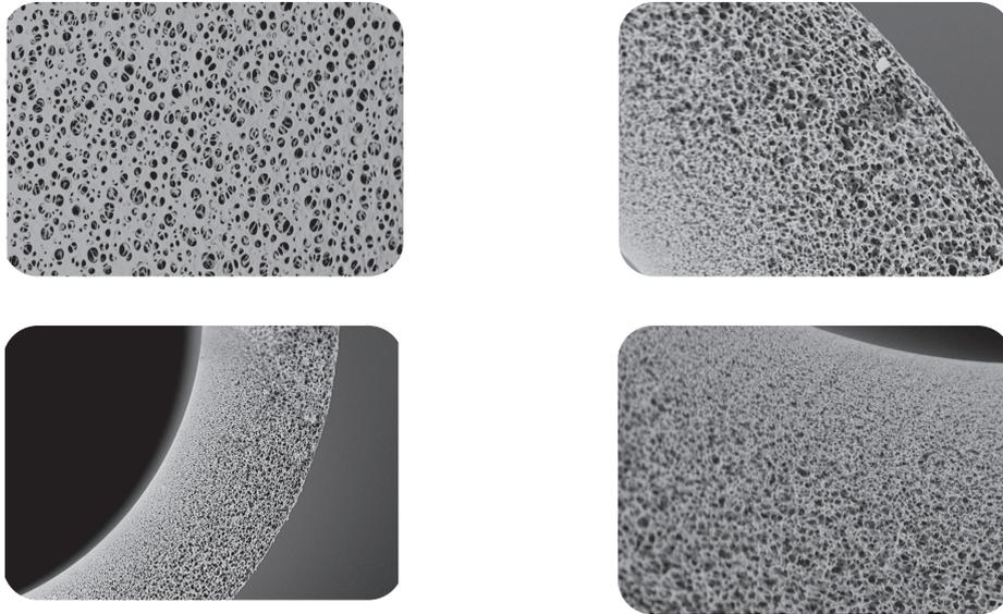
GVS hollow fiber membrane made of modified polyphenol is an asymmetric structure, the membrane layer is dense, and the outer layer is relatively open. Its unique structural design can result in lower bioburden, lower non-specific adsorption, faster filtration rate, higher throughput, and shorter filtration time, so it is very suitable for the pharmaceutical and food industries.
